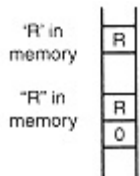
Figure 3.3: This figure shows the difference in memory between 'R' as a character constant and "R" as a string constant.
