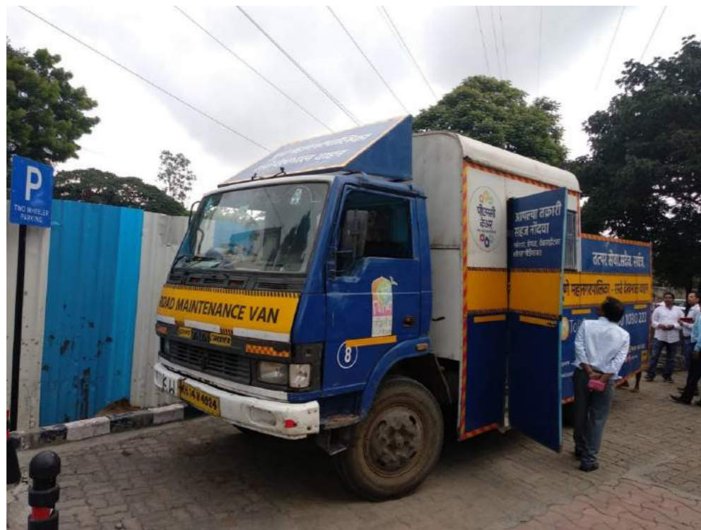
Fig. Pune Municipal Corporation 24x7 maintenance vehicle for quick repair; the van is equipped with bollards, tiles, paver blocks, etc. Citizens can lodge complaints online/ on mobile app and the maintenance van staff fix it.
